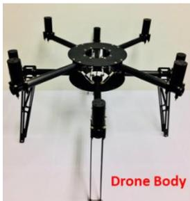
The existing CFRP (carbon fibre-reinforced plastic) drone was brittle at low temperatures and the many CFRP parts were damaged in the event of a collision, resulting in breakage.
