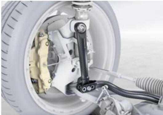
For the first time in a serial-produced car, the stabilizers on the front and rear axles are made of carbon, as well as their coupling rods – all with outstanding performance.
