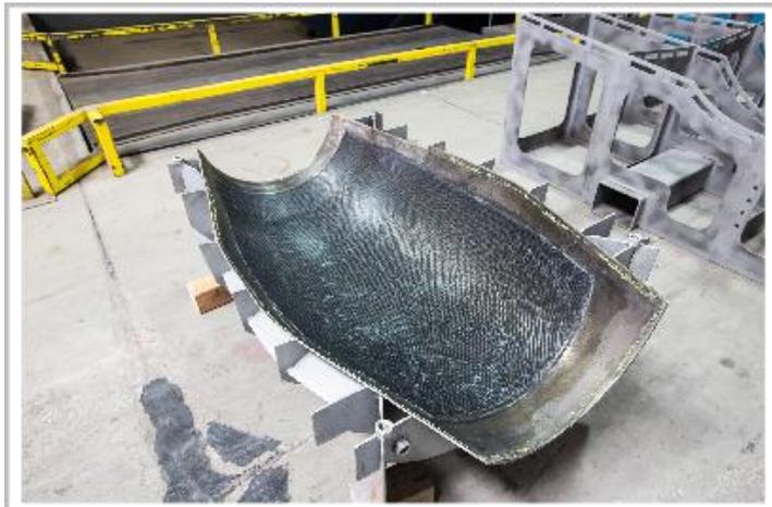
HyVarC® is a patent-pending hybrid InVar and carbon fibre composite layup mould. HyVarC® layup tooling offers a high-precision, lightweight, short lead time solution for prototype and development applications.
