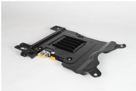
The most important component for vehicle integration of an inductive charging unit is the glass fibre-reinforced plastic (GFRP) holder, which must meet the demanding package requirements while ensuring the charging function and safety. The structural function is ensured by oriented glass fibre reinforcements and ribs formed during the compression moulding process that provide protection against mechanical stress.
