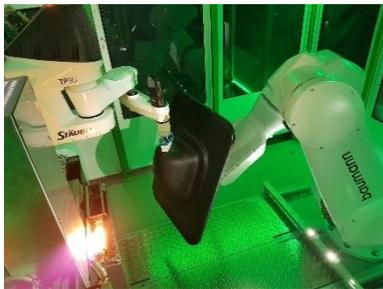
Automated fibre placement (AFP) processes produce a lot of uncured prepreg tape material scrap because all reels of tape are simultaneously changed as soon as the tape left on one reel is not enough to place the next layer of the laminate. With large AFP systems that process up to 32 reels in parallel, manufacturers suffer from high scrap rates of ~10%.
